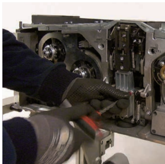
Detail of fast replacement of Welding Group.
