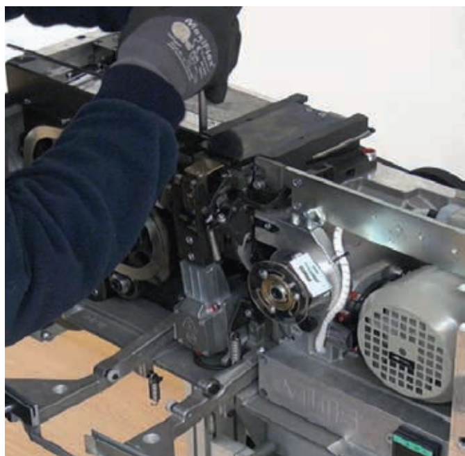
Detail of fast replacement of Clamping Group.
