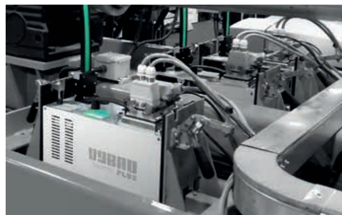
Installation on a vertical strapping machine with press (cardboard application)
